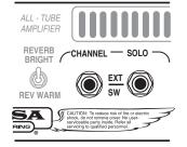
The **EXTERNAL SWITCH** jacks respond to any tip-to-ground latching type logic for their triggering. This type of switching logic can be found on most midi master control switching units on the market.
